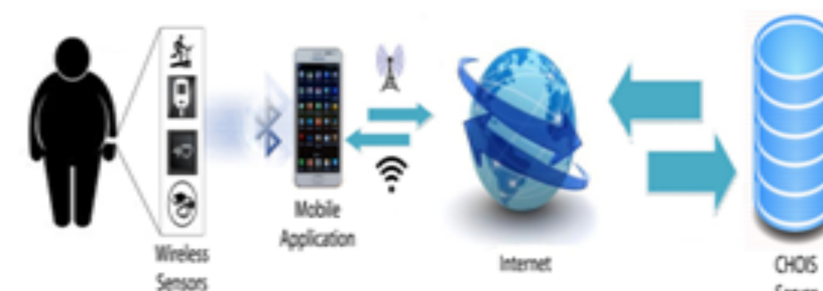
Figure 7. Health-IT infrastructure for collecting real-time streaming physiological data for patient monitoring
